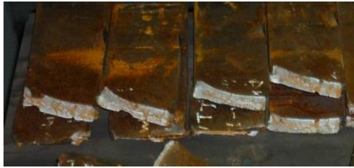
(a) Gull-wing DWTT specimens
