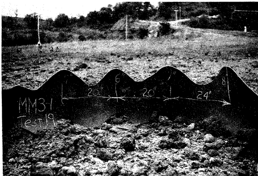
Figure 2.2 Sinusoidal brittle fracture [17]
