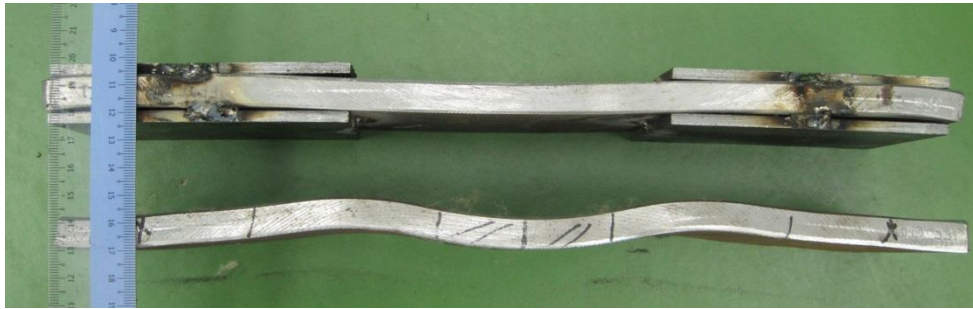
Figure 5.4 Reinforced and gull-wing DWTT specimens
