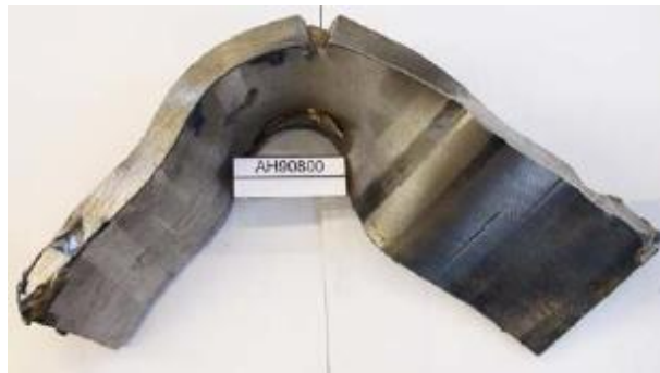
Figure 2.16 ‘No-Break’ specimen extracted from a seamless smaller-diameter pipe [41]
