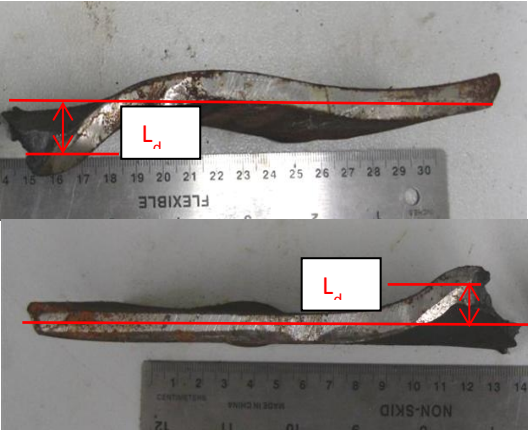
Figure 4.14 L_d measured in gull-wing and flattened specimens
