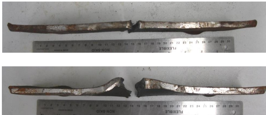
Figure 4.12 API 5L X70 flattened specimens
