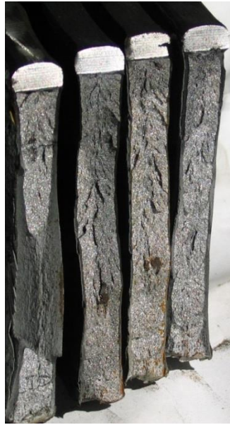
Figure 2.14 Brittle DWTT performance of DN350 12.7 mm wall thickness API X42 PSL2 pipe with an average Charpy energy value over 100 J at 0°C [27]
