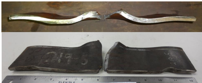
Figure 4.8 Specimen with excessive deformation
