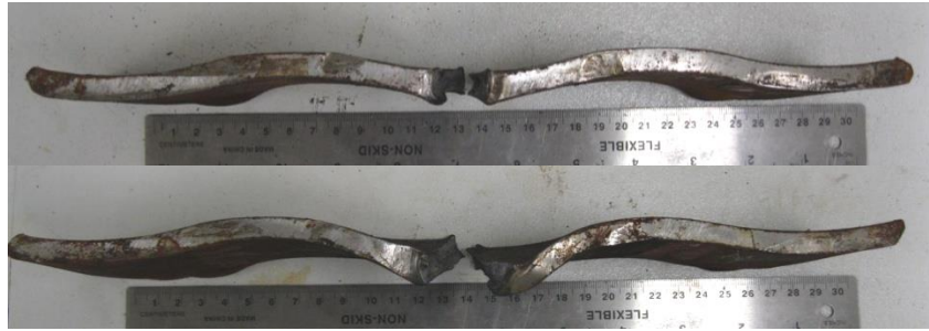
Figure 4.11 API 5L X70 gull-winged specimens
