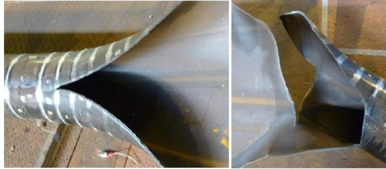
Figure 5.6 Fracture propagation at the pipe body side (left) and seam weld side (right)
