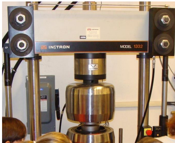
Figure 3.2 Instron model 1332 hydraulic tensile testing machine
