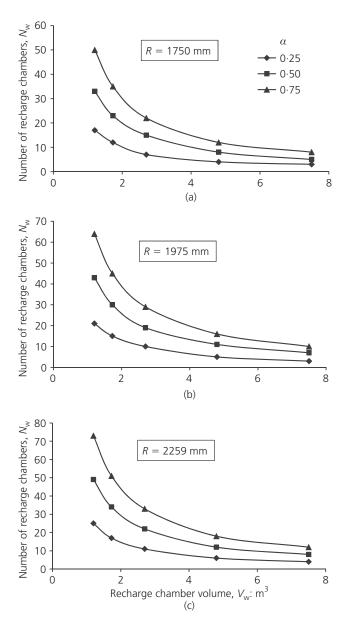
**Figure 9.** Variation of recharge chamber volume with number of chambers for (a) R = 1750 mm, (b) R = 1975 mm and (c) R = 2259 mm
