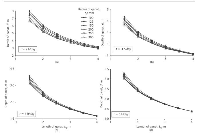
**Figure 6.** Variation of depth of qanat at base versus length of qanat leg for pumping duration (a) t = 2 h/day, (b) t = 3 h/day, (c) t = 4 h/day and (d) t = 5 h/day
