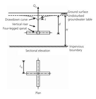
Figure 1. A typical four-legged qanat
