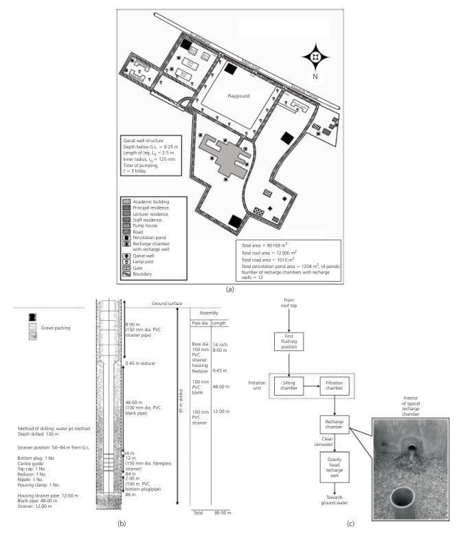
**Figure 10.** Application of proposed technique. (a) Contai Polytechnic campus area showing proposed locations of qanatwell structures, percolation ponds and recharge chambers with recharge wells (not to scale). (b) Cross-section of recharge well adopted. (c) Methodology of recharge through recharge wells and recharge chambers, after Sarkar (2007) recharge through recharge wells and recharge chambers, as per Sarkar (2007), is shown in Figure 10(c).
