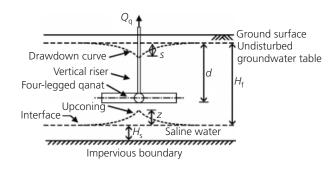
Figure 2. Withdrawal of groundwater by qanat in salinity-affected aquifer
