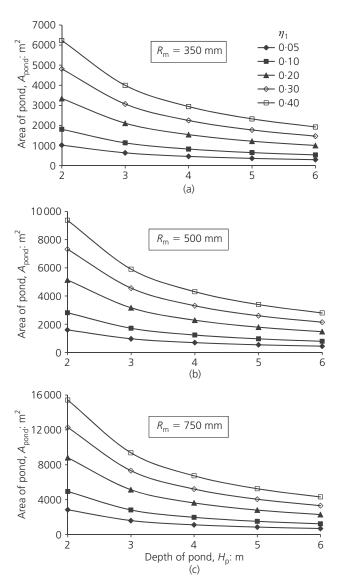
**Figure 8.** Plots of recharge pond area versus pond depth for monsoon precipitation of (a) 350 mm, (b) 500 mm and (c) 750 mm
