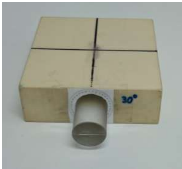
Figure 32: Angular Dependence Jig (The University of Wollongong)
