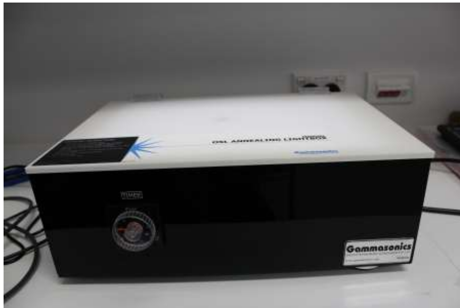
Figure 15: Gammasonics® OSL manual annealing lightbox
