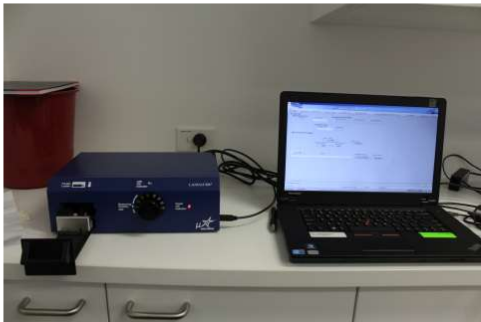
Figure 14: Landauer InLight microStar OSL readout system
