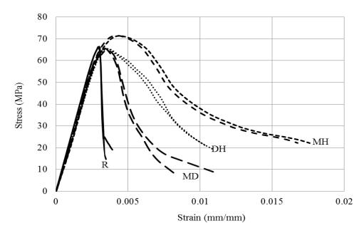
Figure 2. Stress-strain behavior of HSC with and without hybrid steel fibersss.
