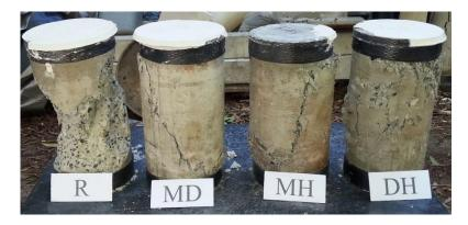
Figure 3. Typical failure modes.
