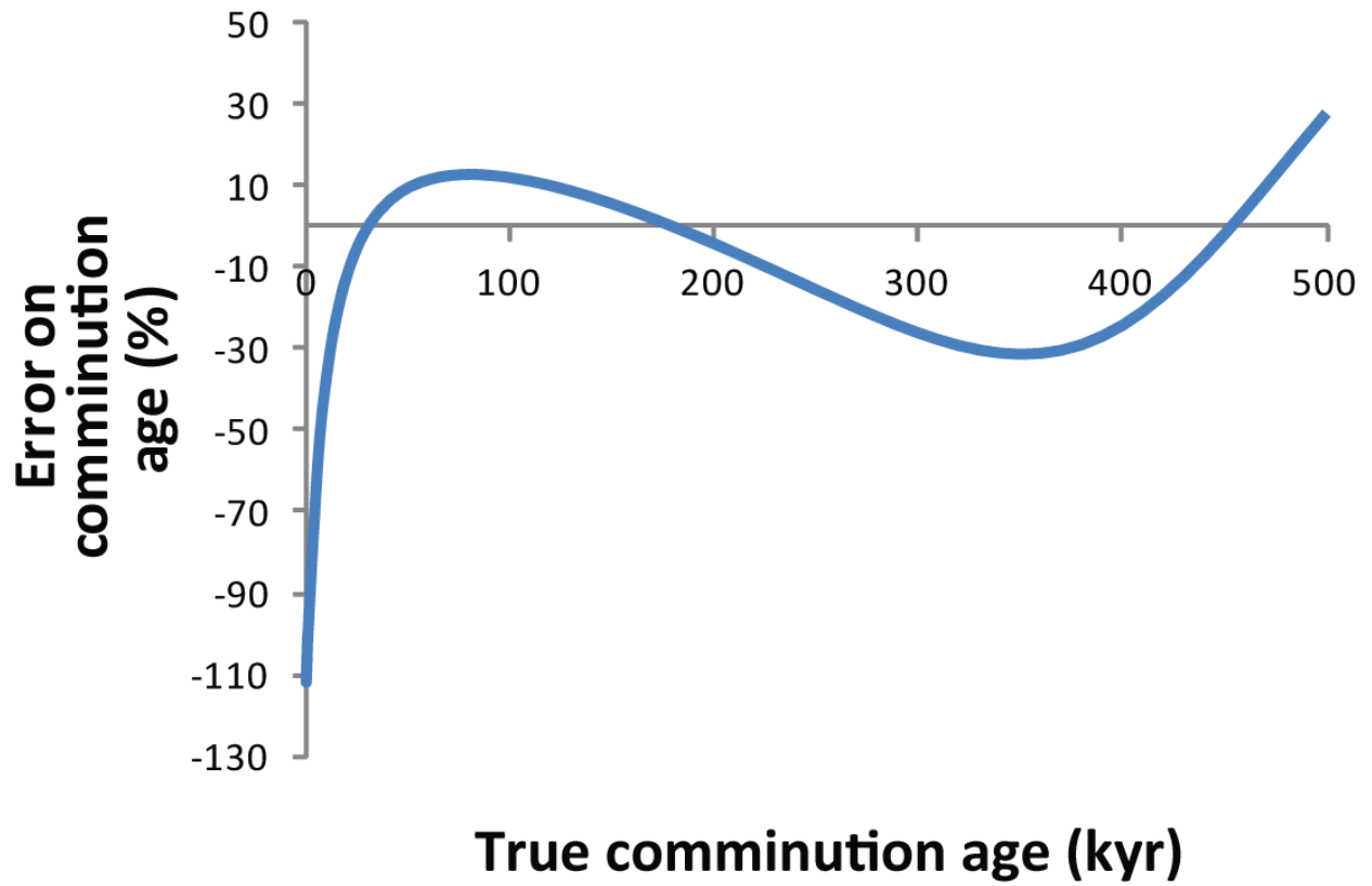
Figure 5. Difference between calculated comminution ages considering a time-dependent f_4 and a constant f_4 , as a function of the true comminution age. See text for details.
