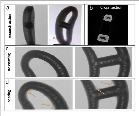
**Figure 4.** MicroCT images of the 3D-printed devices: (a) 3D view and (b) cross-section of the designed cage highlighting the internal porosity. 2D  $\mu$ CT slices for a no coated (c) and coated cage (d). Arrows show presence of POSS-PCU coating.
