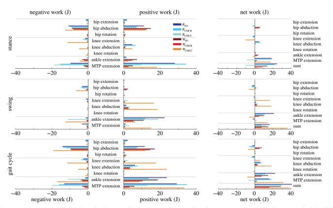
Figure 2. Positive, negative and net mechanical work generated by the reserve actuators in each simulation. Positive/negative work indicates energy (joules) added to/removed from the limb during the movement. Sum: total of all reserve actuators.
