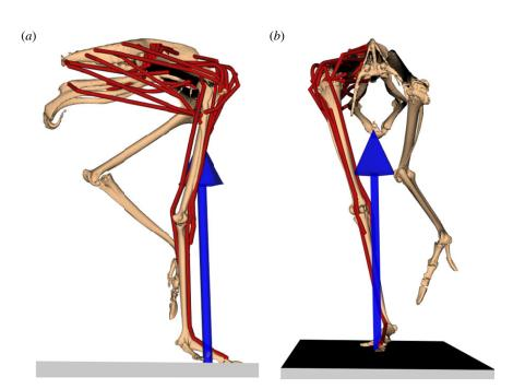
Figure 1. Musculoskeletal model at mid-stance during running. The arrow (blue) indicates the direction and location (centre of pressure) of the ground reaction force. Muscle – tendon actuators (red lines) of the left limb were replaced by idealized joint actuators. (a) Sagittal view. (b) Frontal view.
