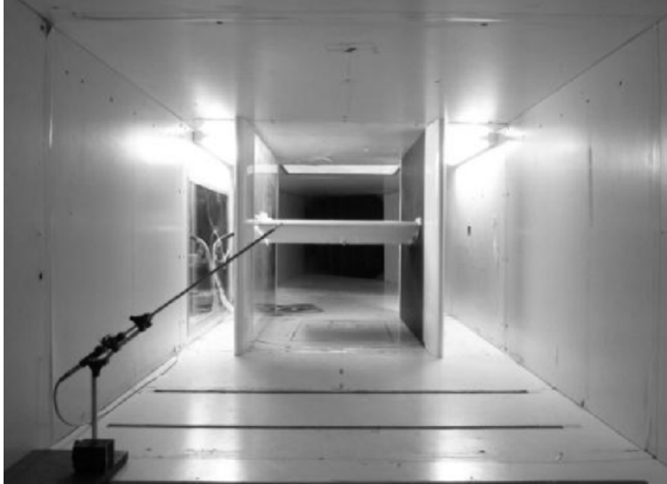
Figure 6. NACA 2212 at wind tunnel section. Source: [8].
