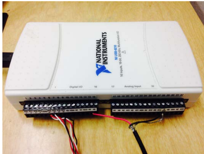
Figure 13. Modified Nikon MC-DC1 hooked-up to Ni USB-6210 digital converter.
