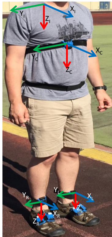
Figure 1. Sensor Mounting Locations along with the Basis Vectors of the Chest, Left Leg, Right Leg, and Inertial Reference Frames
