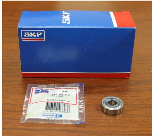
Figure 41. Circular Bearings for Use on Outer Plate and Outer Bracket.
