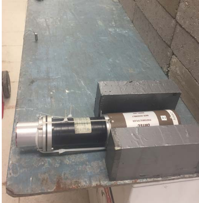
Figure 8. Photo of experimental setup of NE-213 liquid scintillator using a Cf-252 neutron source from a distance of 50 cm.
