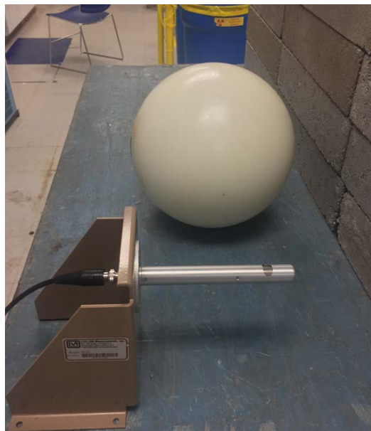
Figure 10. Photo of polyethylene sphere and aluminum tube filled with \text{BF}_3 which were used in this study to acquire experimental data.
