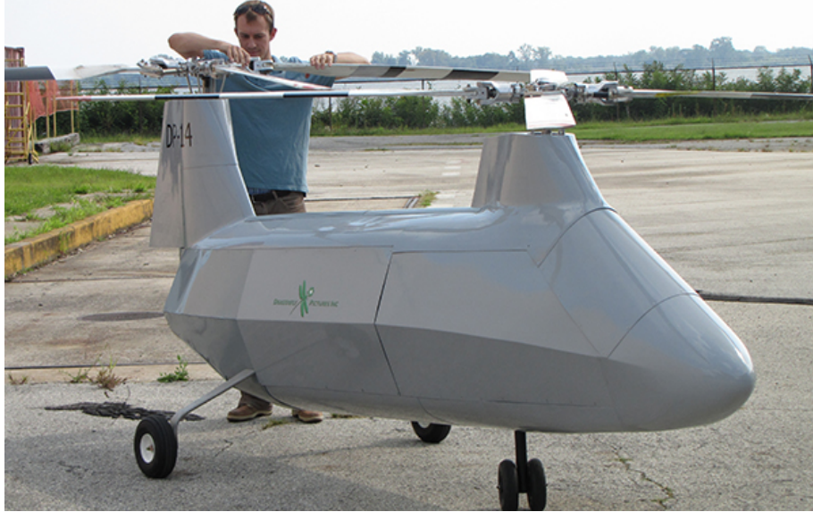
Figure 24. A Worker Installs Rotors on the DP-14 Hawk. Source: DPI Systems (2014b).
