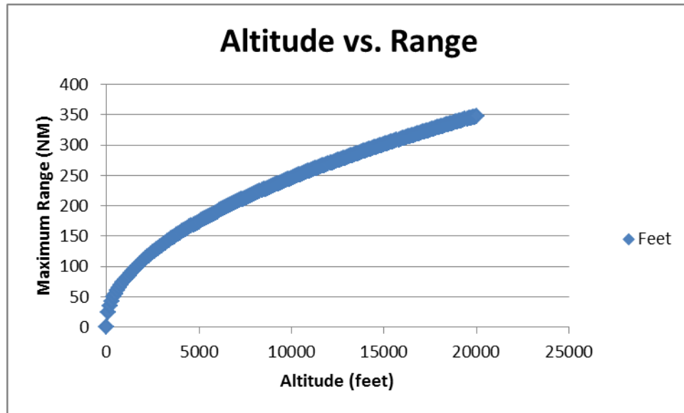
Figure 26. Relationship of Altitude (feet) to Maximum Range (nautical miles) Assuming Co-altitude UAVs.
