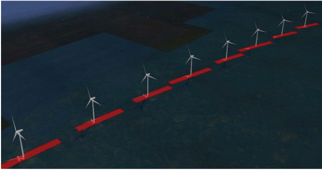
FIGURE 13: Assessment of the potential impact of Middelgrunden offshore wind farm (Denmark) on fictitious shore-based VTS radar. Red areas over the sea surface represent the clutter that the turbines would generate on the radar display [24, 25].
