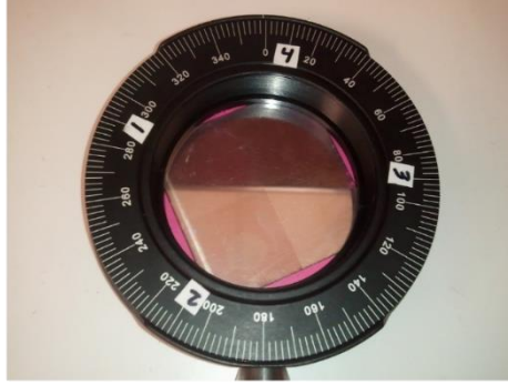
Fig 4-26: Fabricated wire grid polarizer mounted in an optical rotation stage. Acknowledgement to John R. Middendorf.
