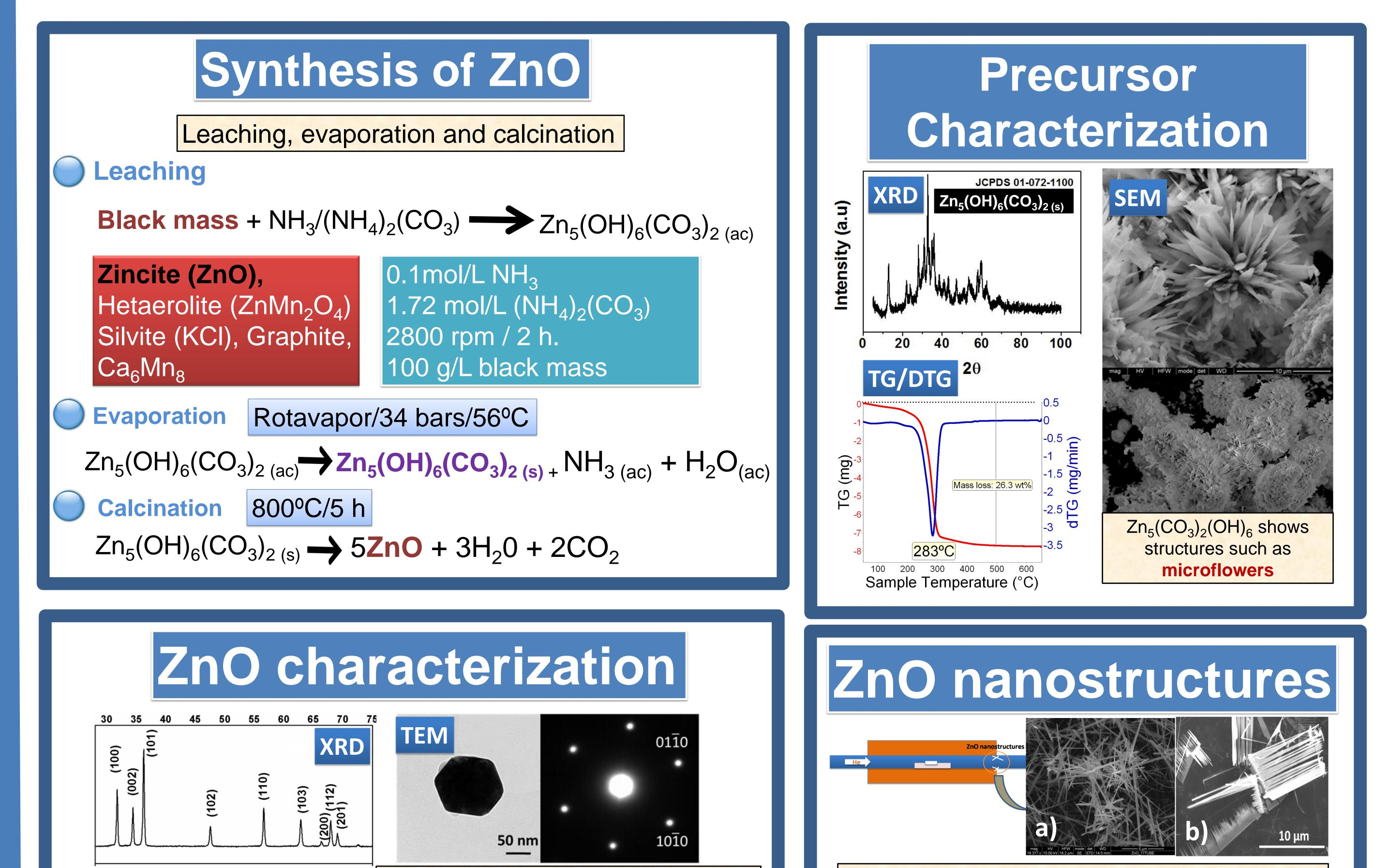
Nanocombs (a) and nanobelts (b) were obtained at lower temperature due to the thermal gradient of the furnace and were extracted from scratching the tube walls.
