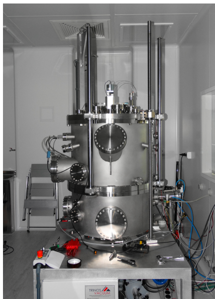
Fig.1. 75-cm diameter, 100- cm height deposition chamber.
