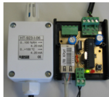
Figure 2: photo about SCRIED design and the temperature and humidity sensor
