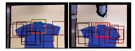
Figure 1. Bounding boxes and FINDDD selected grasping point. The red box contains the collar and FINDDD scores will be calculated inside it.
