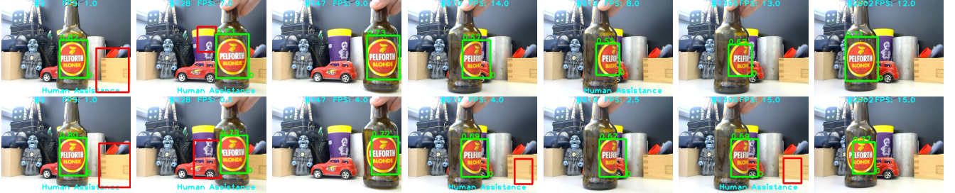
Fig. 6. Detection results for a single object. Top Row: Detection outputs of the proposed method. Bottom Row: Outputs of the approach proposed in [26]. Green rectangles indicate object hypotheses whereas red ones are background hypotheses labeled by the user during the assistance.
