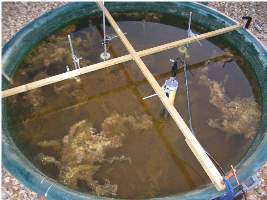
Fig. 2.4. Photograph of the YSI600XLM dissolved oxygen sensor deployed in the centre of the mesocosm.
