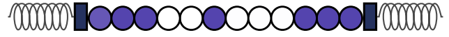
FIG. 12. Illustration of the system with elastic walls with the spring constant k .
