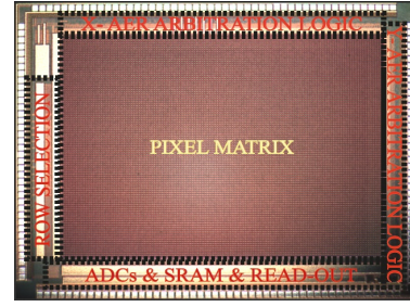
Fig. 4. Sensor's microphotograph. The main system blocks have been highlighted. Chip dimensions are 4.1mm \times 3.3mm.
