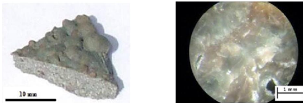
Fig. 4. Glass-ceramic V1 before and after polishing (single view and optical microscopies).
