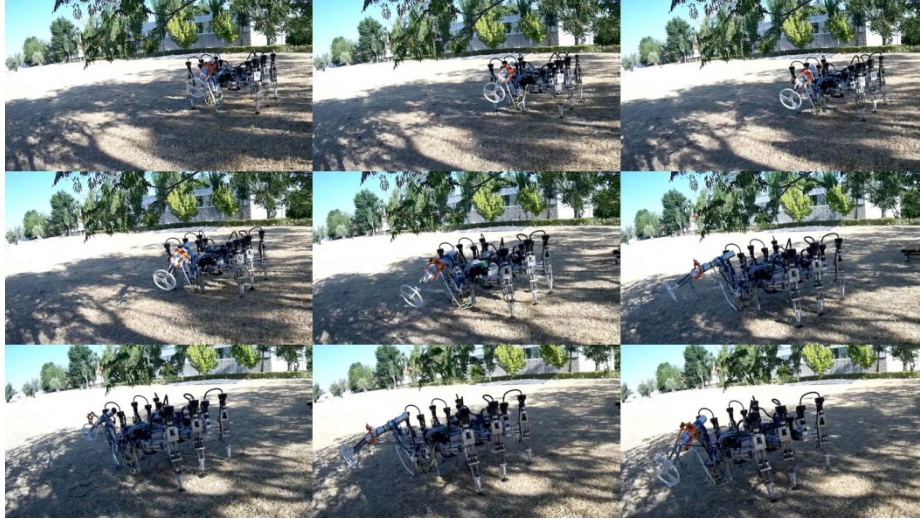
Fig. 10. Photographic sequence (left to right and up to down) of a gait pattern of the all-terrain hexapod robot.
