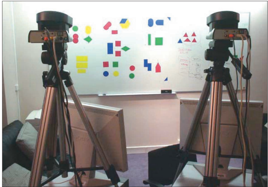
Figure 2. Setup for the Talking Heads experiment. Two pan-tilt cameras look at a white board containing colored geometric figures, which the robots use as subjects of a guessing game.
