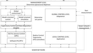
Figure 3 Software and RTC. Adapted from [2]
