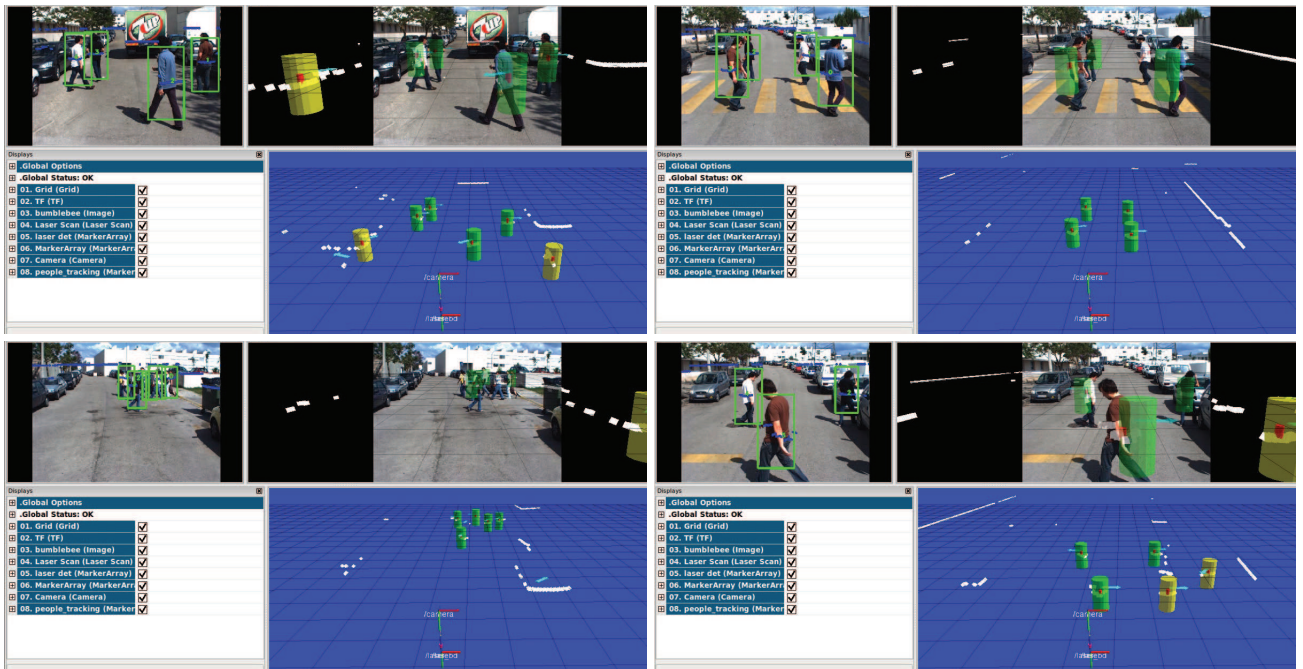
Figure 8: People detection modules output using our feedback-fusion approach from ISR-UC-implidar-sync database. Green cylinders and big green bounding boxes are the people detections results by our fusion approach, respectively. See text for details.
