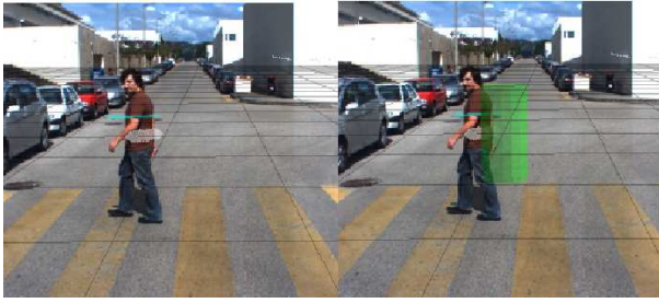
Figure 6: Example of detection using fusion with temporal information. Left Image, image without the temporal information used as feedback. Right image, image with the temporal information used as feedback. The right image shows that the person has been correctly detected.
