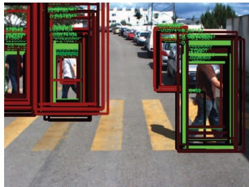
Figure 3: Image detector. The score of the detections are represented by their bounding box color: green represents very high score, black medium score, and red very low score.
