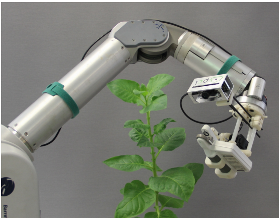
(b) Object-related task setup: ToF camera attached to a manipulator end-effector, in this case a Chlorophyll meter, to get measures by touching the leaf surface.
