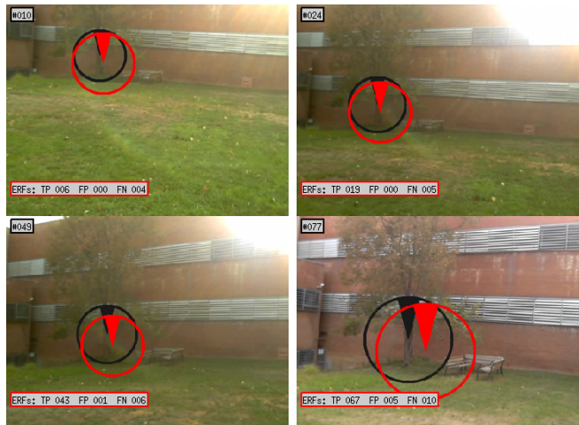
Fig. 11. 3D target detection. Our approach is able to learn and detect 3D targets in outdoor environments. Red circle indicates the classifier output, whereas black one is the ground truth or visual target.
