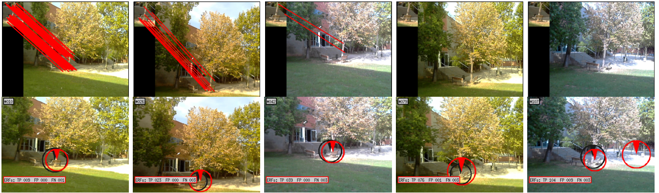
Fig. 2. Failure of keypoint-based methods. Top: Matching of SIFT features (red lines) between the visual target (small top-left image) and a sequence of image examples that includes lighting and viewpoint changes. Bottom: Output of the proposed detection approach (red circles) for the same target and sequence. Black circles indicate the ground truth and the rectangle shows the detection rates: true positives (TP), false positives (FP) and false negatives (FN).
