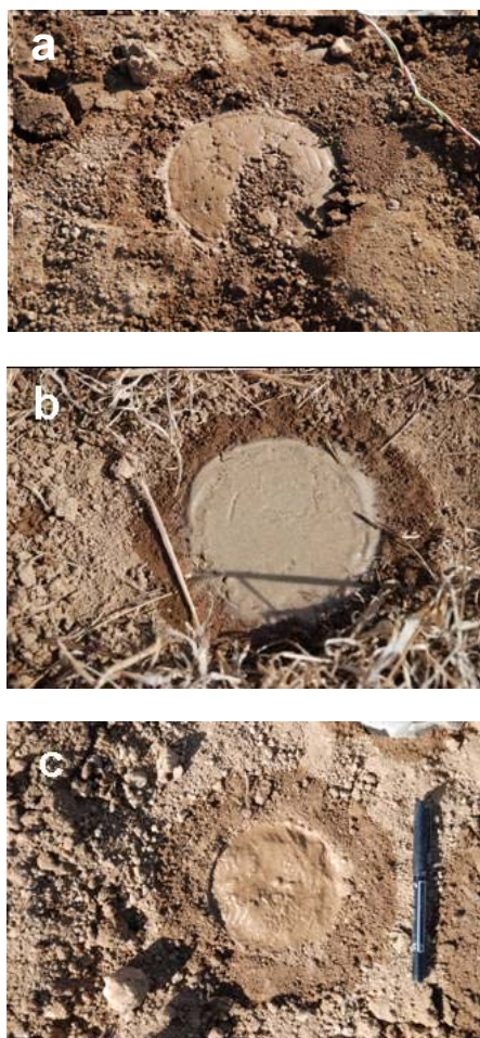
Fig 7. Soil surface at the end of an infiltration experiment after removing the conventional plate (a) without and (b) with a contact sand layer, and (c) after removing the malleable disc base
