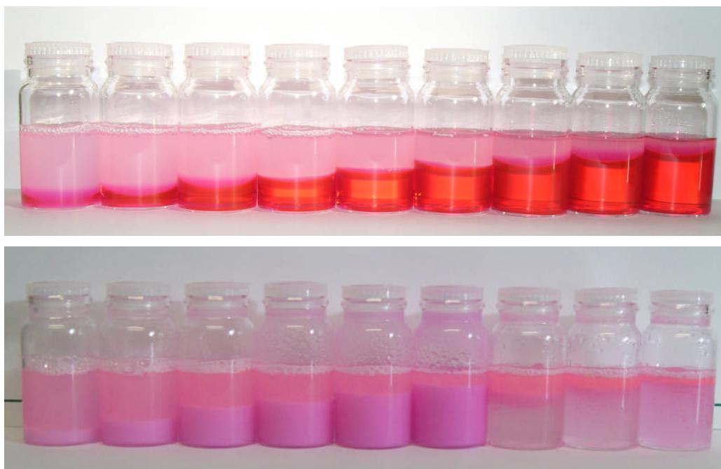
Figure C-5. Styrene monomer and fumed silica HDK H2000 aqueous dispersion (initially dyed in red with rhodamine): Before and after emulsification by hand-shaking, top and bottom respectively. W/o emulsions were obtained up to 60 vol% of water.
