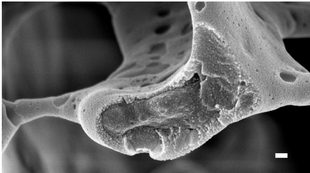
Figure VI-4. Cryo-SEM image of nanocomposite polymer foam obtained after freezing a mixture of a PVL latex and Ludox silica nanoparticles at -210\text{ }^{\circ}\text{C} with silica/polymer ratio and total solids content (wt%) of 0.38 and 13.0, respectively. The image was taken after full sublimation of the ice. Scale bar 200 nm.
