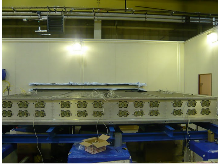
Figure 2.17: Photograph of a tracker ECal module during construction. The front-end electronics boards can be seen mounted on the module side.
