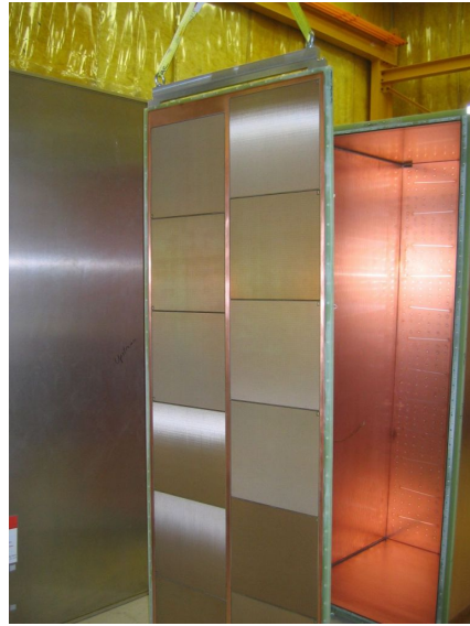
Figure 2.15: Photograph of a TPC during assembly.
