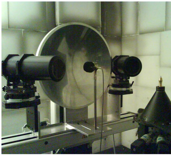
Figure 8.2: Acoustic mirror, near focus microphone and traverse arrangement
