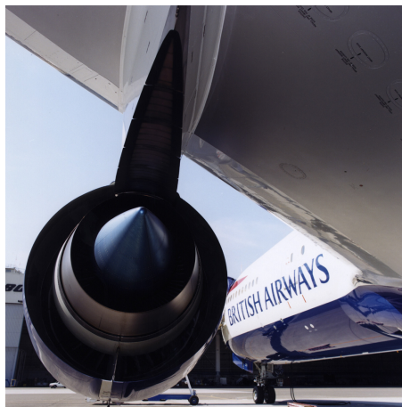
Figure 2.1: Rolls-Royce Trent 800 engine on a Boeing 777 ( photograph is reproduced with the permission of Rolls-Royce plc, copyright Rolls-Royce plc 2006 )
