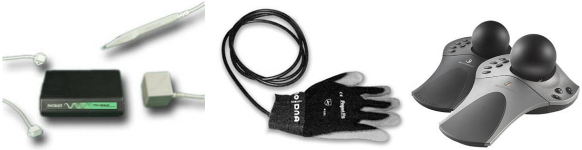
Figure 2.8: VR Input Devices (from left to right): Motion Tracker, Data Glove, Space Ball
