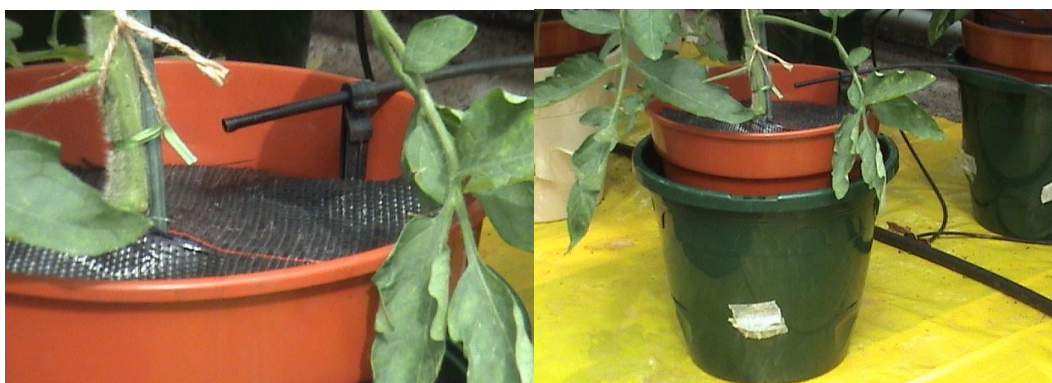
Figure 4.3. Plants were grown in 9 litre pots covered with Uvi matting to minimise evaporation. Pots were placed in a container which acted as a reservoir to allow accurate measurement of the volume of drainage water.
