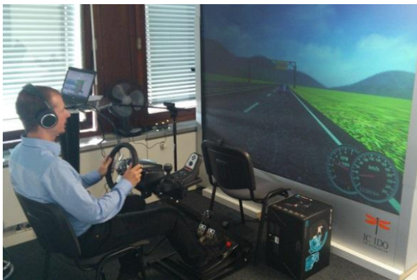
Figure 2. Driving simulator setup.
