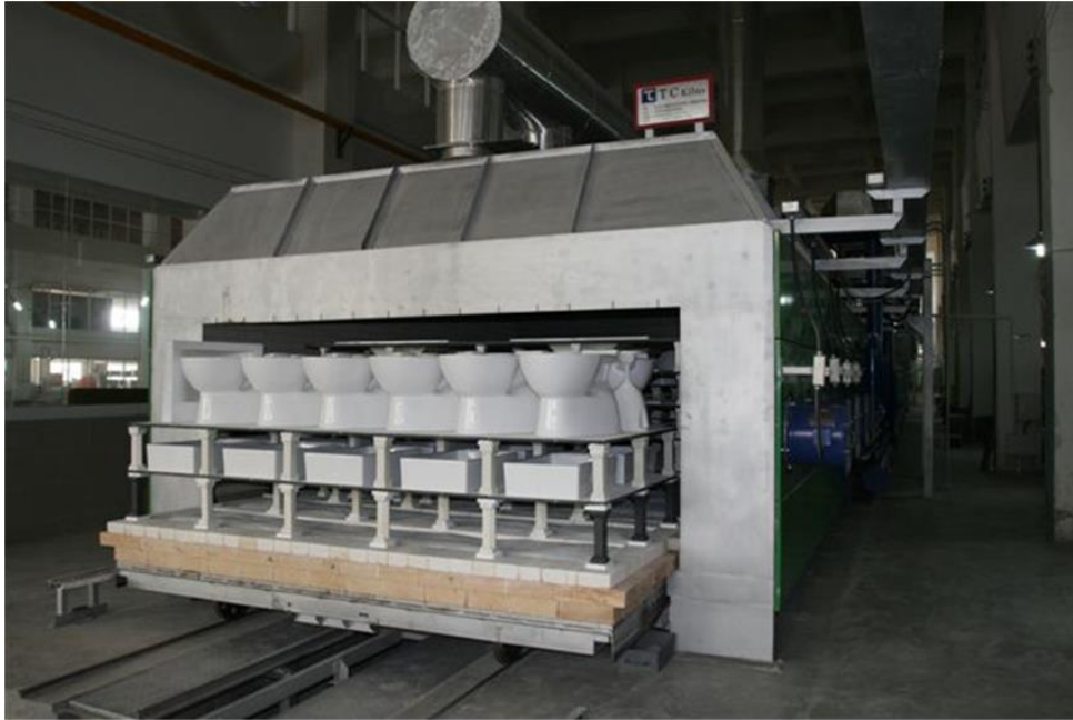
Fig. 5.2.1.9: Kiln aggregate in a sanitary ceramic industry. Tunnel aggregate with long sintering times.
