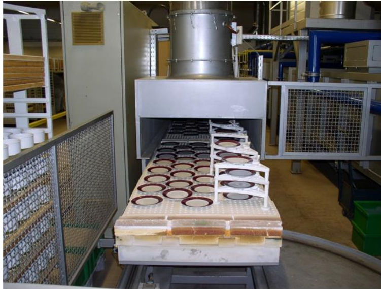
Fig. 6.2.7: Firing of ceramic decoration.
