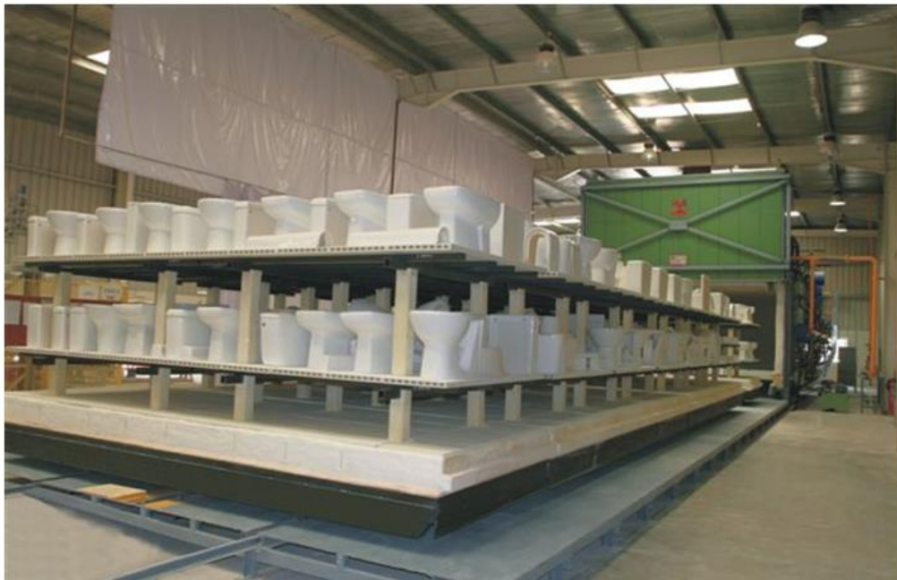
Fig. 5.2.1.10: Kiln aggregate in a sanitary ceramic industry. Bogie hearth kilns with shortened sintering times.
