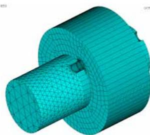
*Longitudinal pin connections for transmission of torque as an alternative to feather key connections are little applied in industrial practise. At the Institute of Mechanical Engineering investigations of the dynamic load-ing are executed.*
