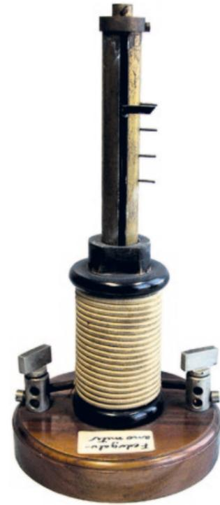
Abb. 38: Federgalvanometer.
