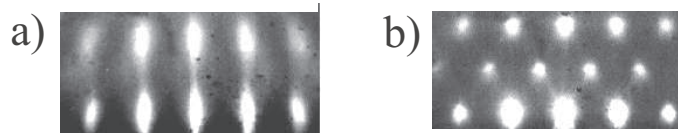
Figure 4.24: a) The RHEED transmission pattern obtained from a lightly sputtered Nb(001)-surface. b) RHEED-transmission pattern originating from a Pd film of 20 ML thickness deposited on Nb(001). This diffraction pattern occurs typically with the epitaxy of late transition metals and noble metals on open (001)-surfaces of cubic substrates. In the two cases (a,b) the incident beam was parallel to the [011]-direction of the Nb(001)-surface.
