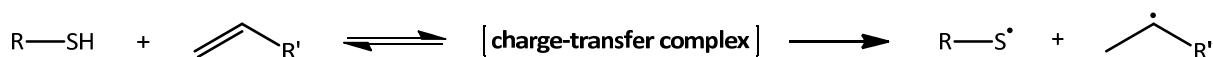
Scheme 5: Spontaneous formation of a charge-transfer complex between an ene and a thiol yielding radicals that unintendedly initiate polymerisation
