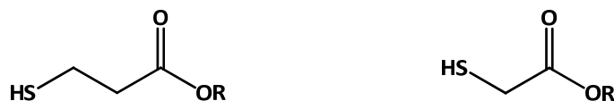
Fig. 9: Molecules frequently used as thiols in TEP; left hand side: mercaptopropionates; right hand side: mercaptoacetates
