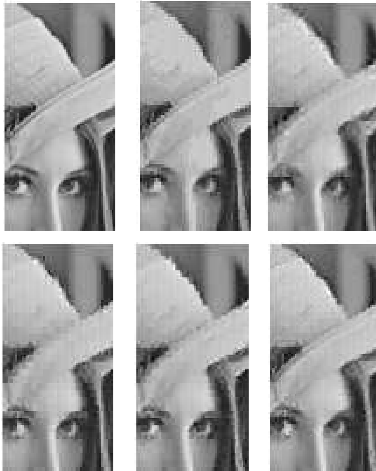
Figure 4.9: Detail of Lena image: original (upper left), and compressed image using 1.25 bpp and neural gas (upper middle), global PCA (upper right), and local PCA by means of VQPCA (lower left), MoPPCA (lower middle) and matrix NG (lower right), respectively.
