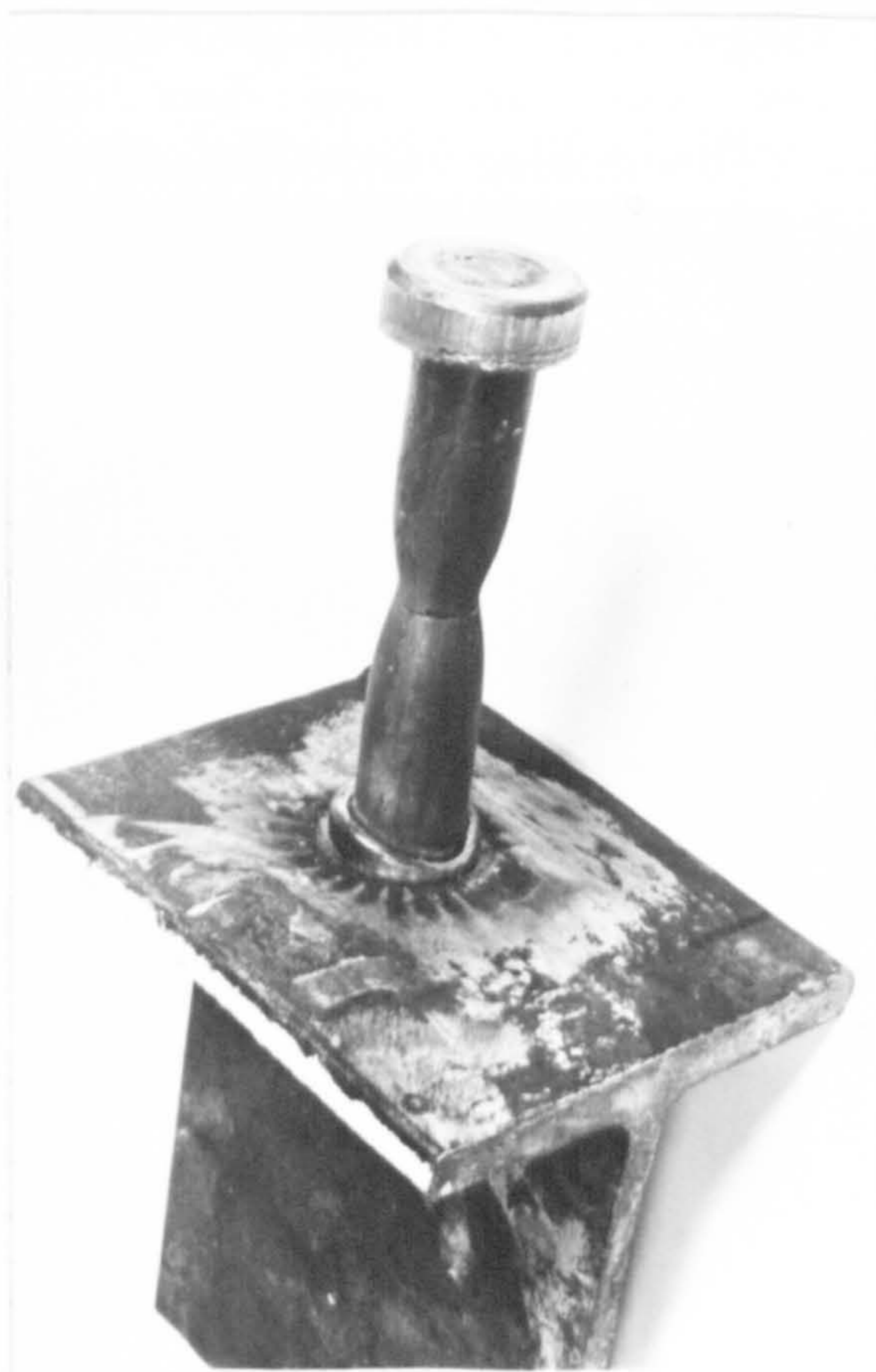
Fig. 5.15 Tensile test on a welded stud.
