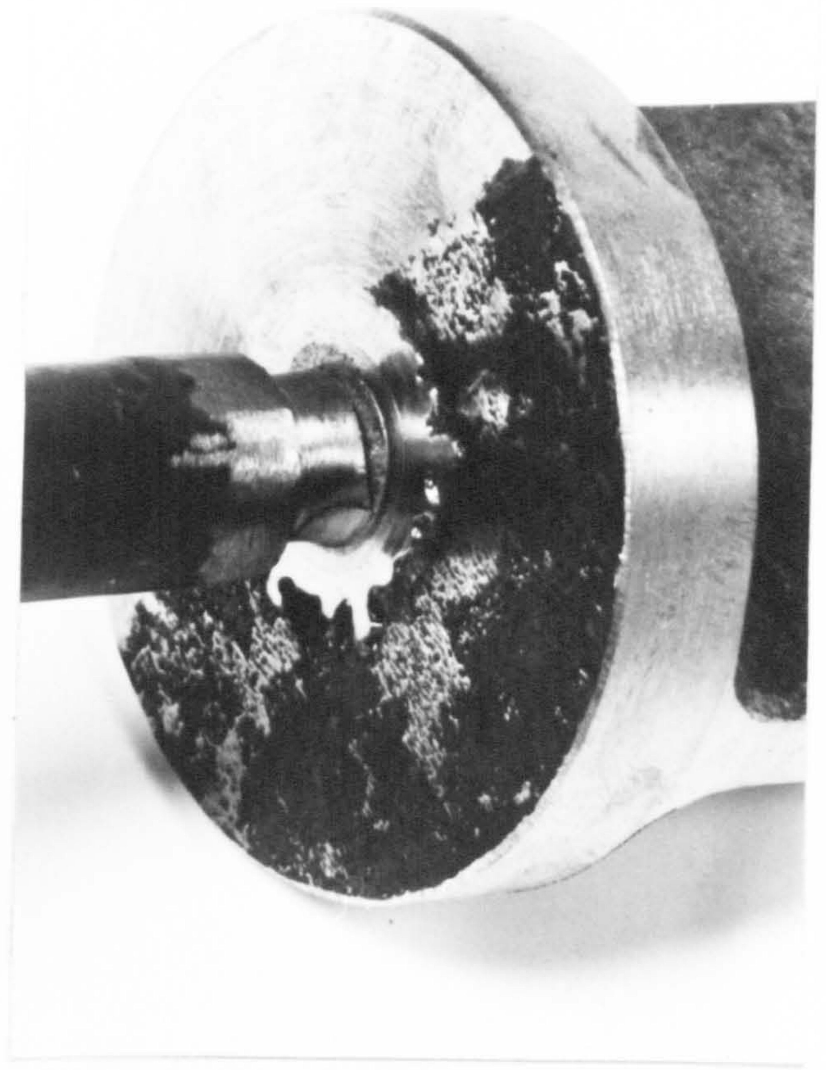
Fig. 5.21 Tensile test on the weld material.
