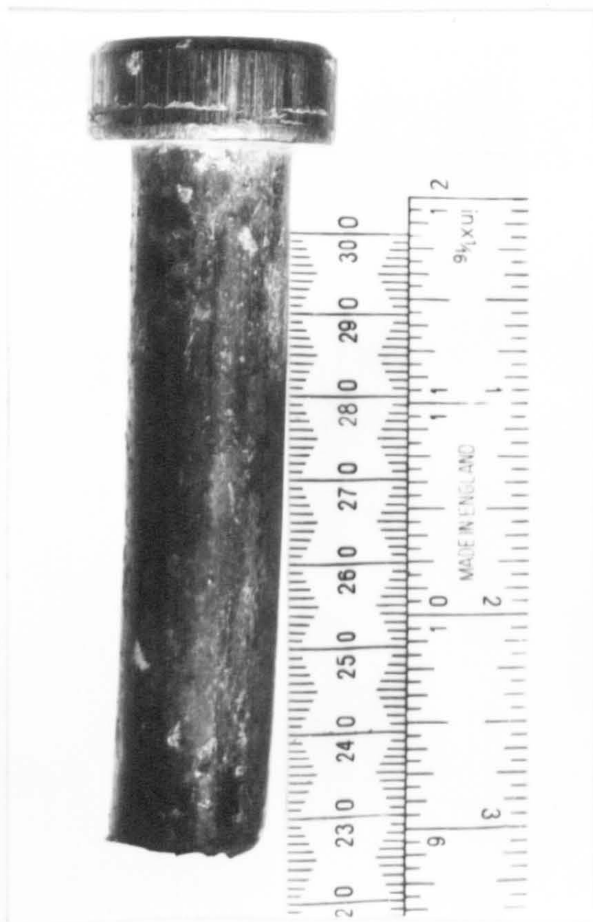
Fig. 5.8 The shank after failure.
