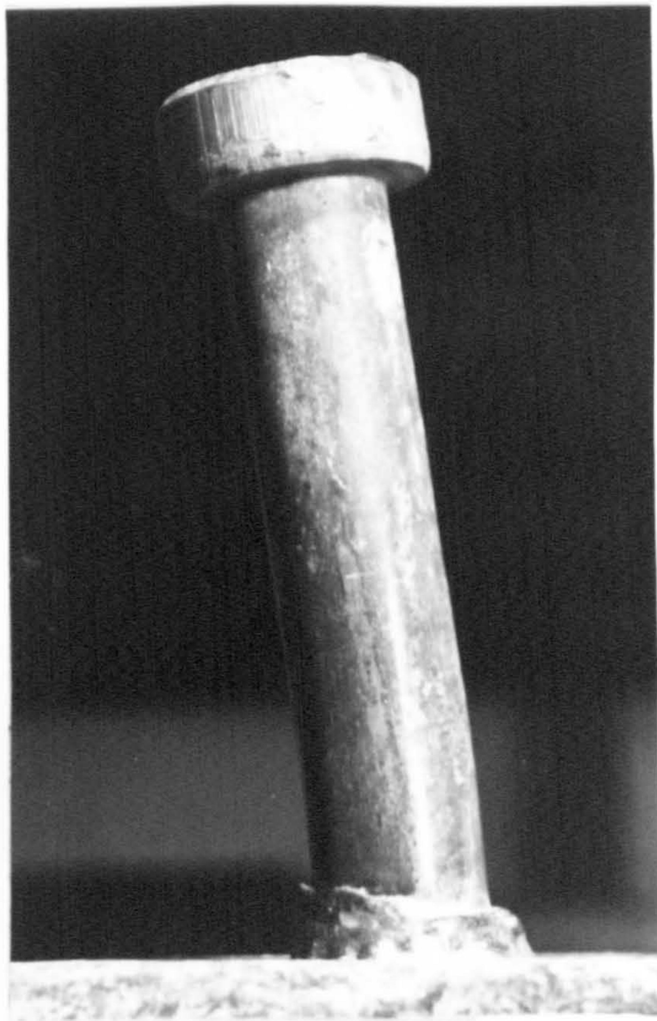
Fig. 5.9 Variation in the height of the weld-collar.
