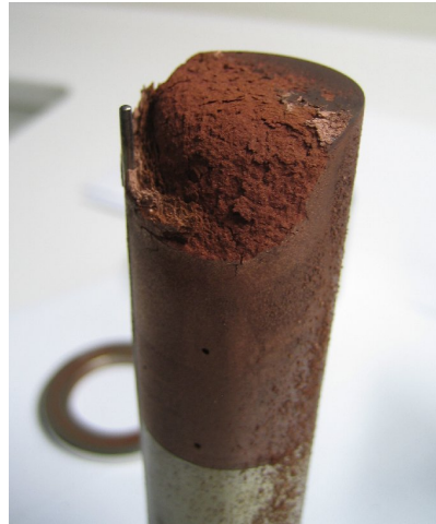
Fig. 35. The core of the heat load probe after runaway impact [98].
