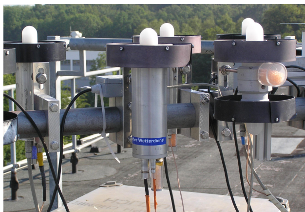
Figure 1. Impression of filter radiometers operated side by side during the ACCENT intercomparison (Bohn et al., 2008).
