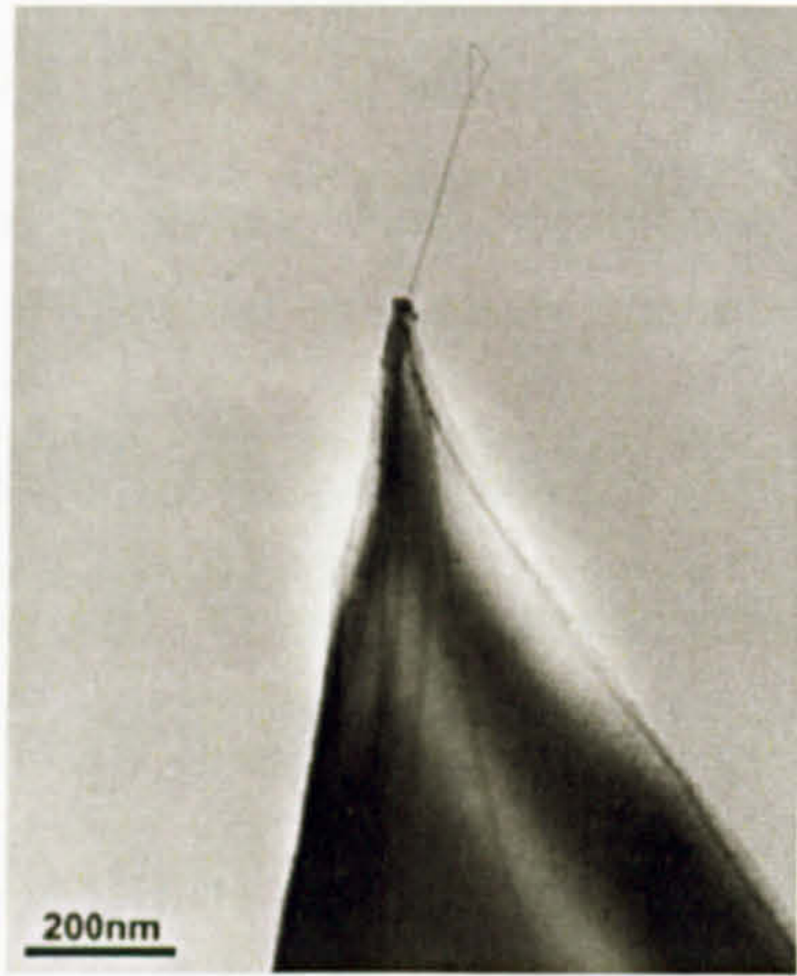
Figure 4.1: TEM image of a SWNT-AFM tip fabricated by cCVD growth directly onto the Si tip. Thanks to Steve York for help with the TEM
