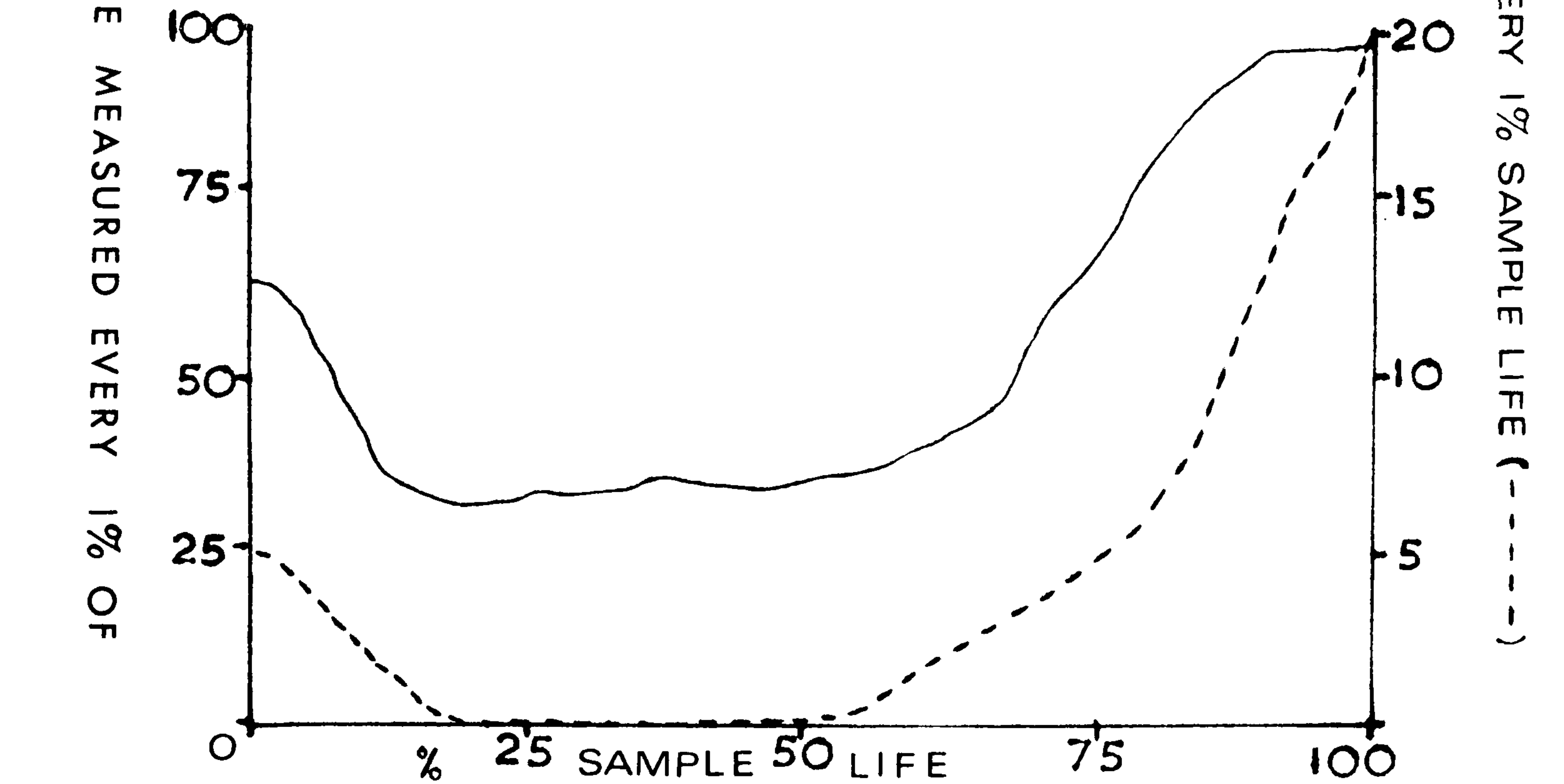
FIGURE 16 : Shows the change in response of an aluminium rod against % fatigue life for the 2-peaked loading spectrum.
