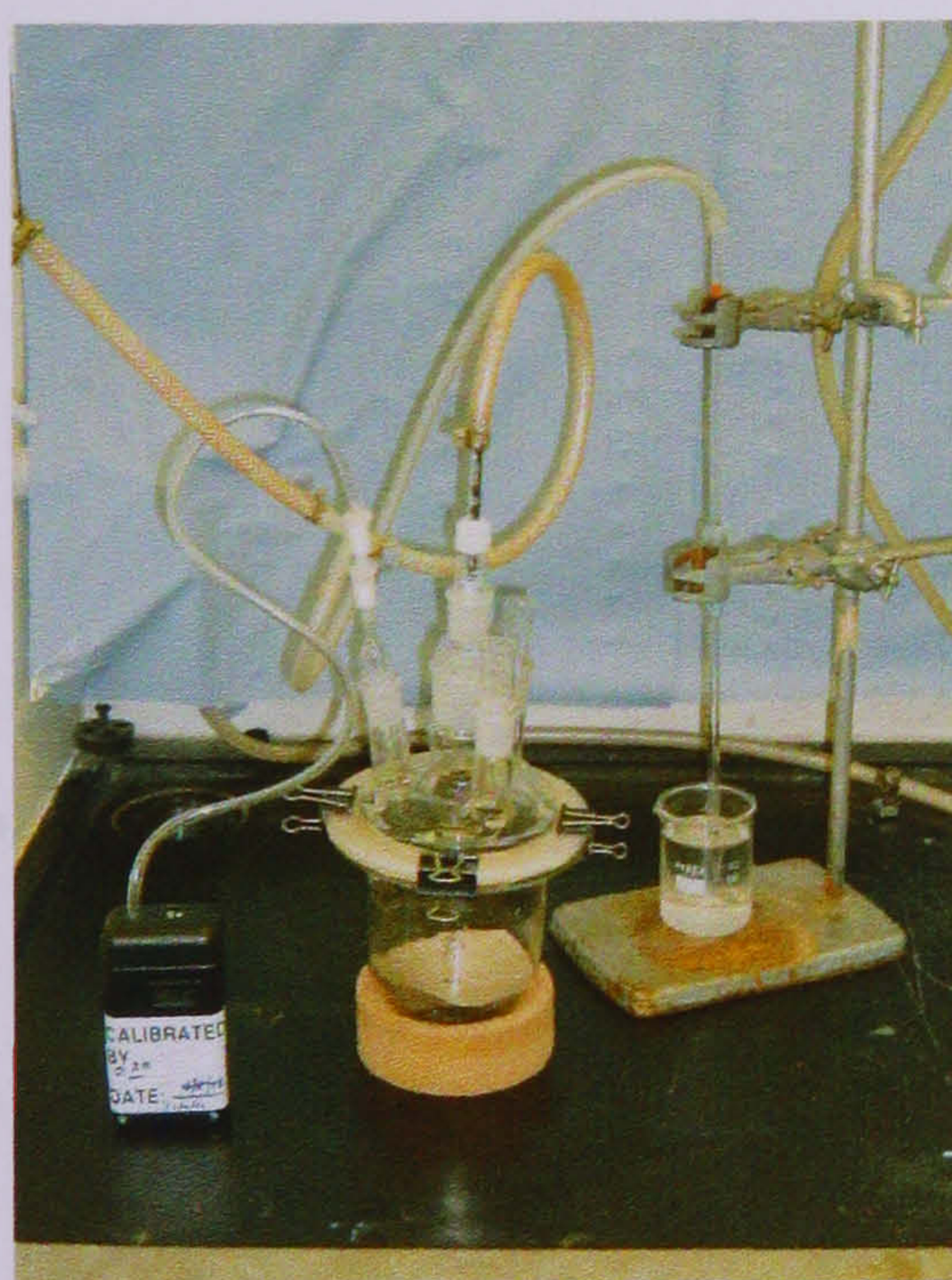
Figure 2.1 Apparatus for generating a test atmosphere: (a) schematic; (b) image of equipment; (c) detail of the aldehyde containing vial.
