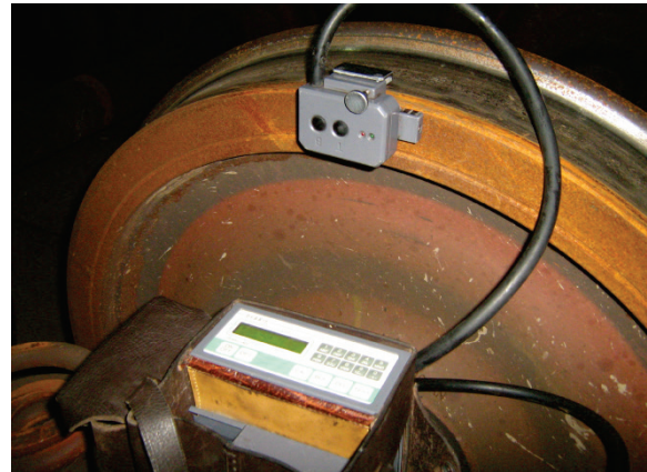
Figure 2 Measurement of residual stresses with DEBBIE machine [7]
