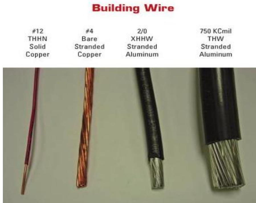
Figure 1. Solid and stranded conductors
