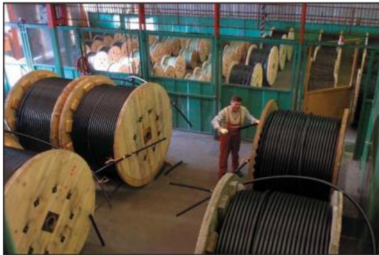
Figure 44. Wooden drums for cables
